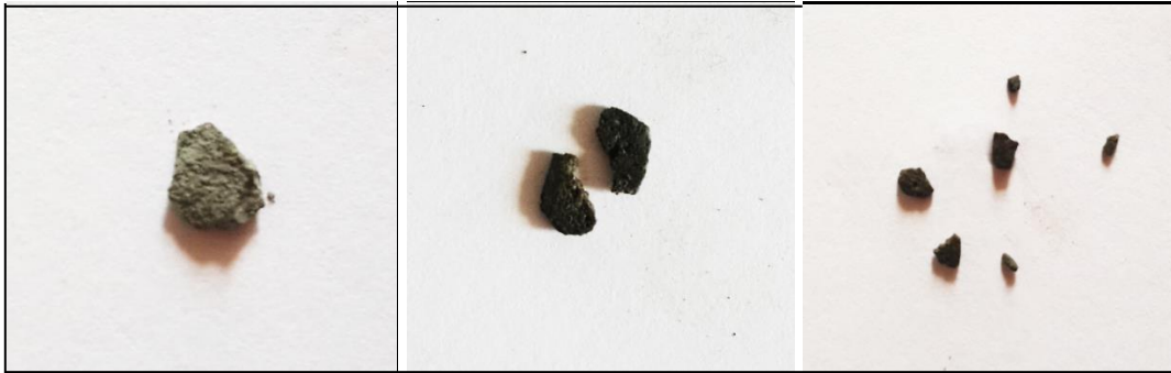
Figure (6): Complete fragmentation of artificial stone by Nd: YAG laser using 19 pulses; each of (2.5 \times 10^{11} \text{ w/cm}^2) in water.
