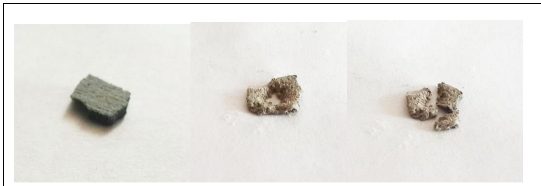
Figure (5): Complete fragmentation of artificial stone by Nd: YAG laser using 200 pulses; each of ( 2.5 \times 10^{11} w/cm 2 ) (in air).
